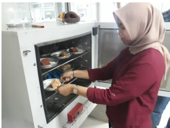
Gambar 4. Preparasi sampel XRD
