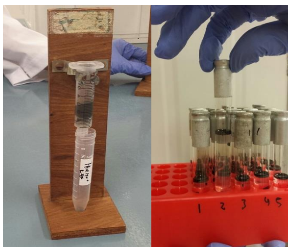
Figure 1. Leaching column for bioleaching experiment (left) and tubes prepared for enumeration of iron oxidizing bacteria (right)
